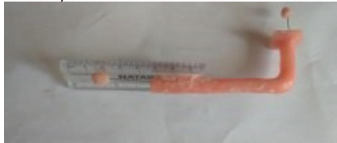
Figure 1: Customized instrument used to measure LTF
